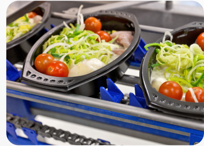
Chain with pegs for processes that require specific reliability.
