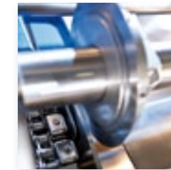
STRIP CUTTING Perfect cutting of film with powerful suction to prevent accumulation of residual strips
